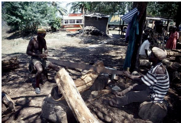
Hand sawing mpingo logs at Sameja sawmill in the Lindi region of Tanzania
